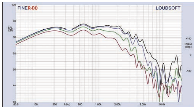
Figure 30: TB Speaker W8-2314 woofer on- and off-axis frequency response (black = 0°, blue = 15°, green = 30°, purple = 45°)
